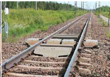
Wheel profile measurement system installed in the southern part of the Iron Ore Line
